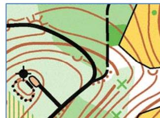
Figure 3: Orienteering map section printed with the CMYK offset printing method, optimised with a stochastic raster
